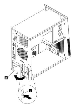
Figure 11. Opening the PCI card latch
